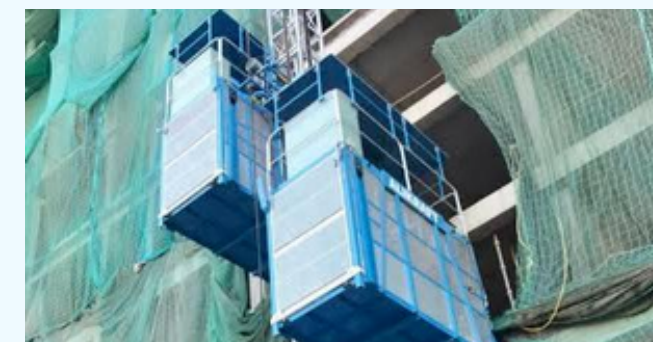
Passenger Service Hoist
